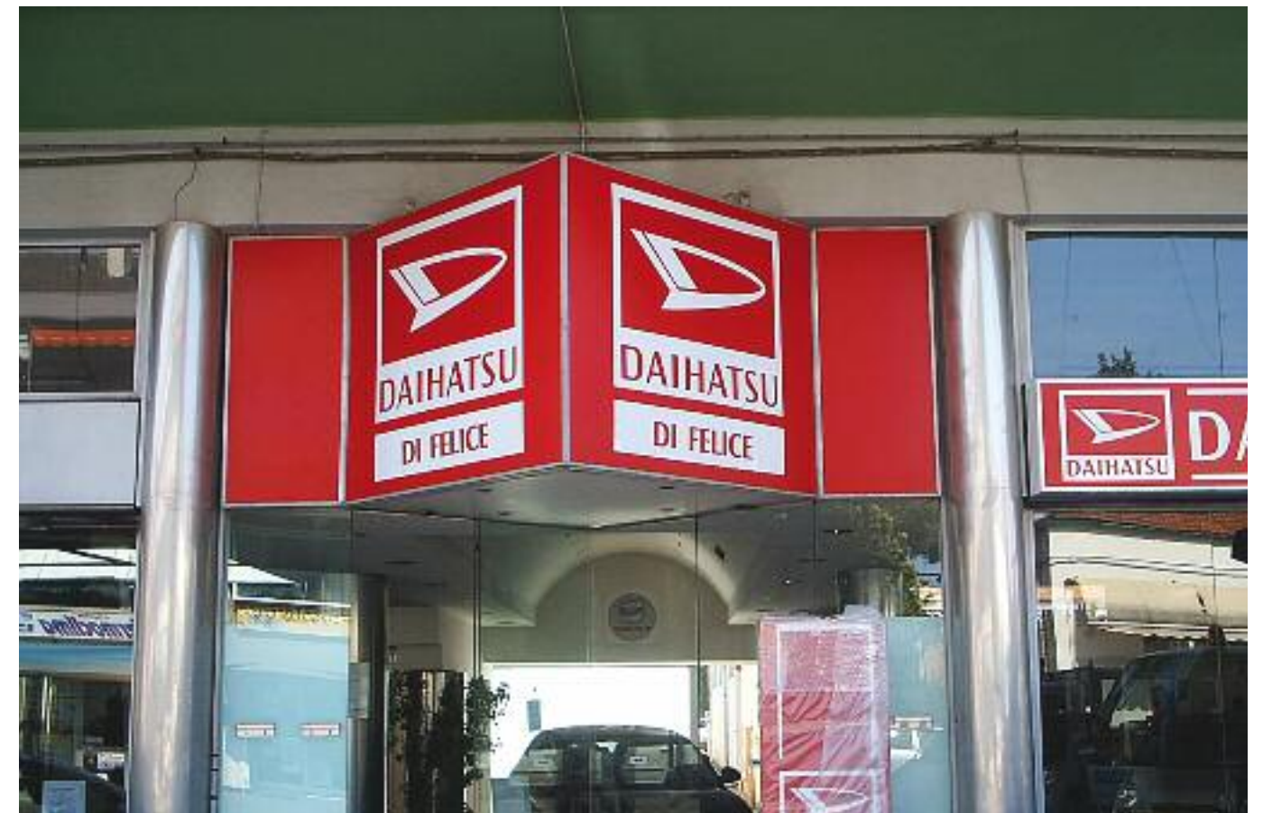
Insegne luminose con diffusore in metacrilato decorate con pellicole viniliche Illuminated signs with methacrylate diffuser decorated with vinyl films
