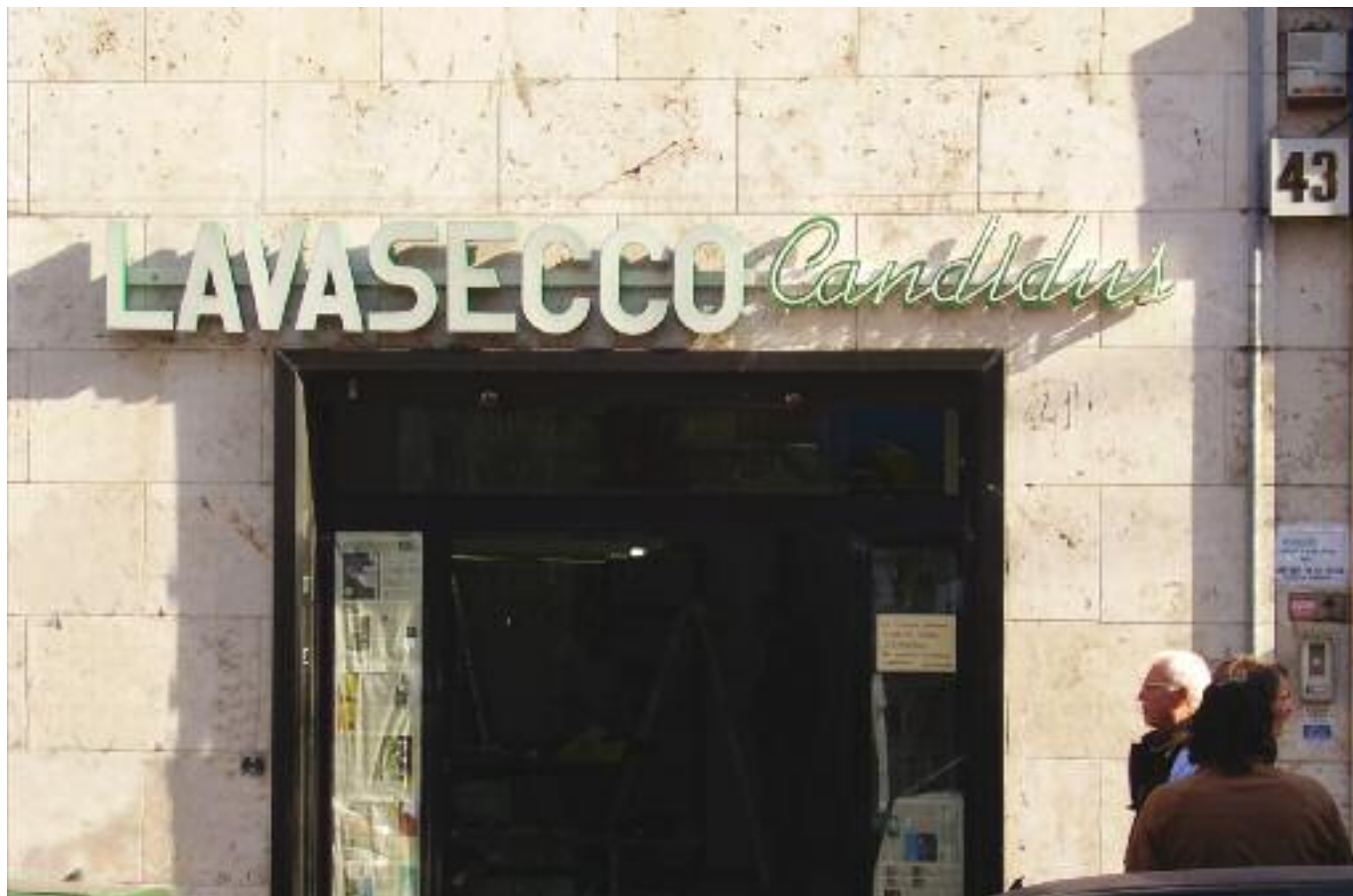
Insegne luminose a lettere scatolate in plexiglass fissate a parete Plexiglass channel letters illuminated fixed to the wall
