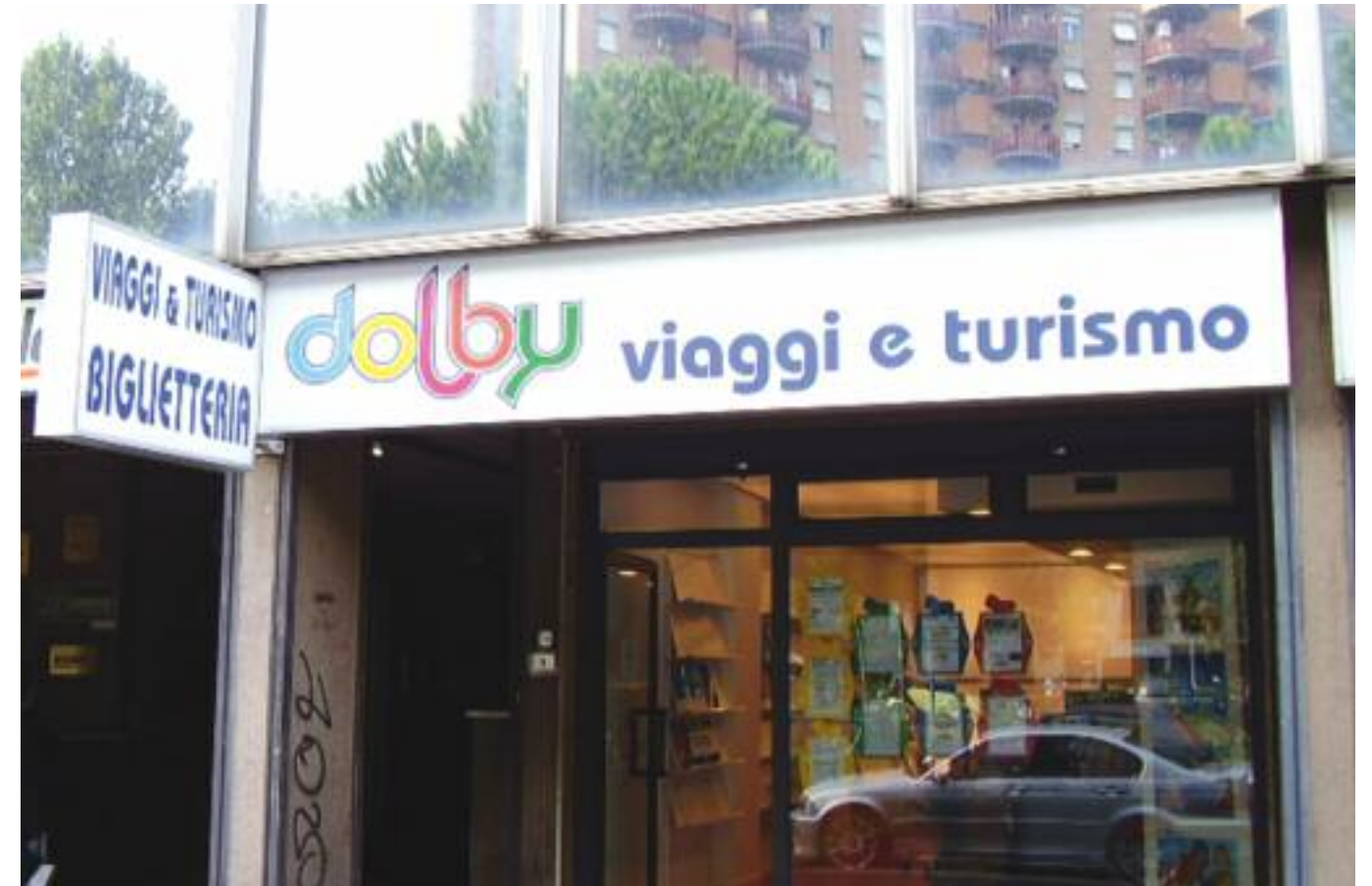
Insegne luminose con diffusore in metacrilato decorate con pellicole viniliche Illuminated signs with methacrylate diffuser decorated with vinyl films
